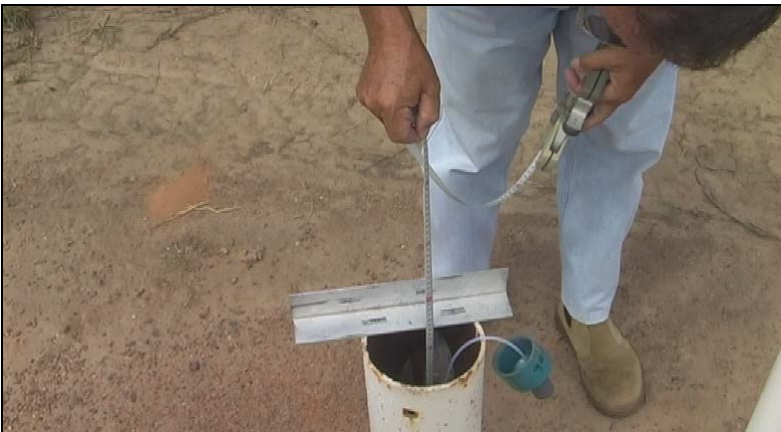
Figure 17: Bore being measured with plover
