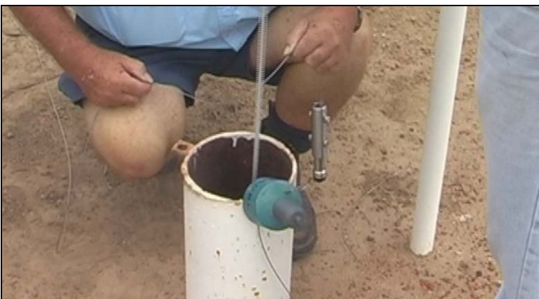
Figure 18: Stainless steel cable attached to diver and bore cap
