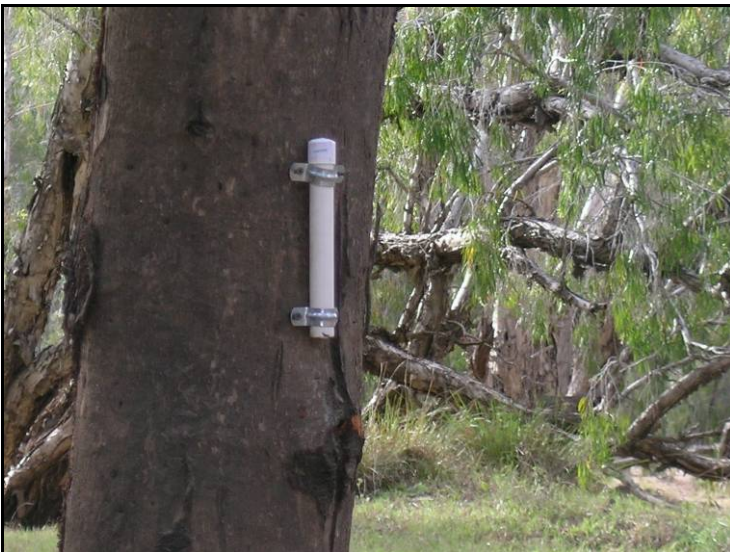
Figure 14: Alternative approach to logger installation (cont.)
