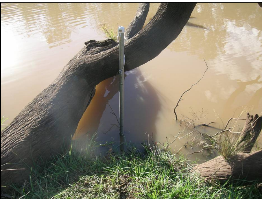
Figure 12: Alternative approach to logger installation
