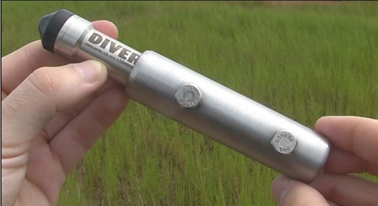
Figure 16: TD Diver with stainless steel weight attached (Note the two attachment points for the diver and the steel cable)
